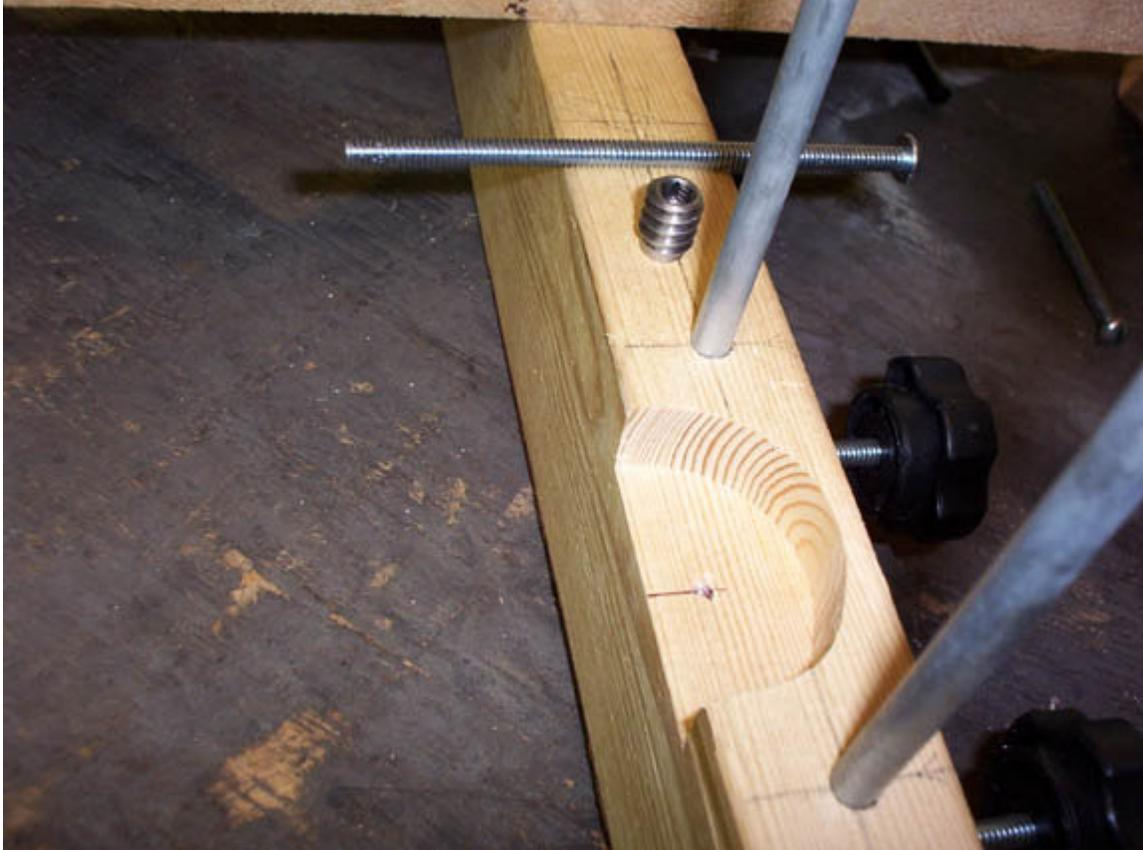
**Now for the threaded inserts that I'm using it takes a 3/8" hole, so using the drill press again, I drilled a hole at least 2" deep just in case I later decide to use longer threaded rods. You'll probably have to move the support rods in order to use the drill press.**
