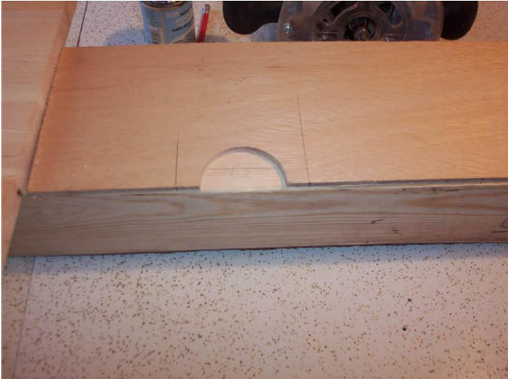
**After the first dial indicator recess was routed out, I made a mark 3/4" away from the 3rd hole from the board and placed the dial indicator recess jig so that the left edge of the circle touched it. Double stick taped it down again with another 2x4 past it to hold the template flat and routed out the second recess.**
