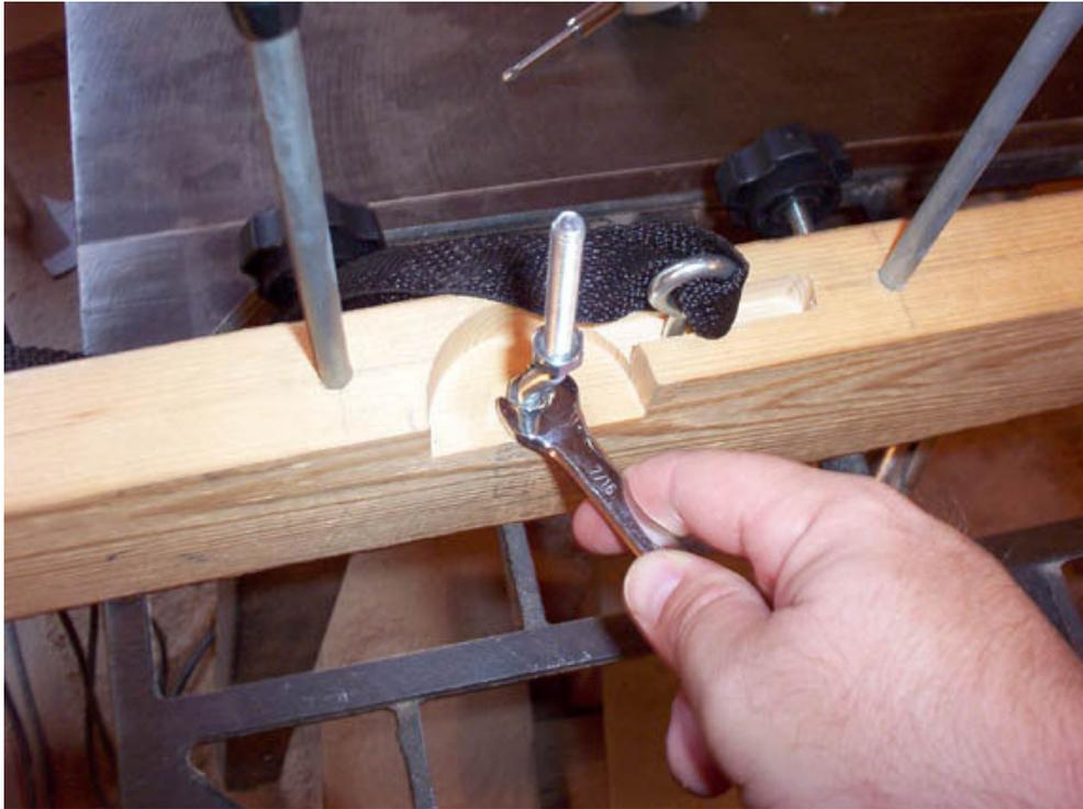
**Now to hold the dial indicators in place all I did was use two 1/4" nuts on both sides of the mounting bracket to hold it wherever it needs to be. It's easy to move it up and down now by moving the nuts up or down. You'll have to experiment to get the proper placement depending on which guitar your jigging. It doesn't take long to figure out though, and making mental notes of where it was, for a particular style guitar, helps also.**
